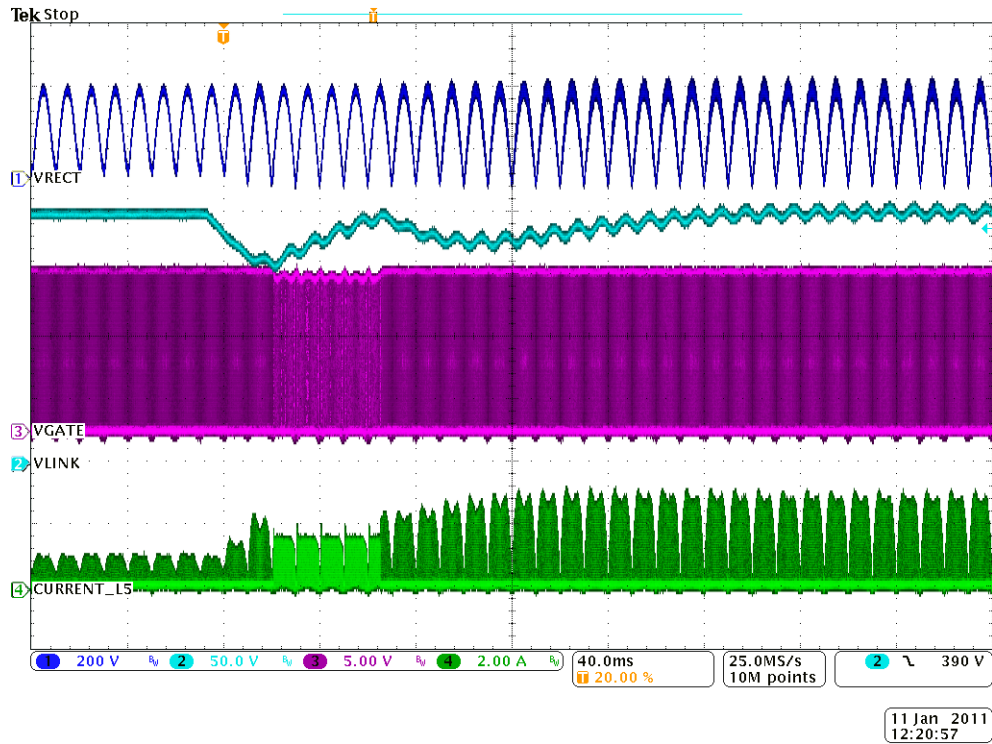
Figure 18. Load Transient — 9 W to 90 W, 1 W/uS, 220 VAC
